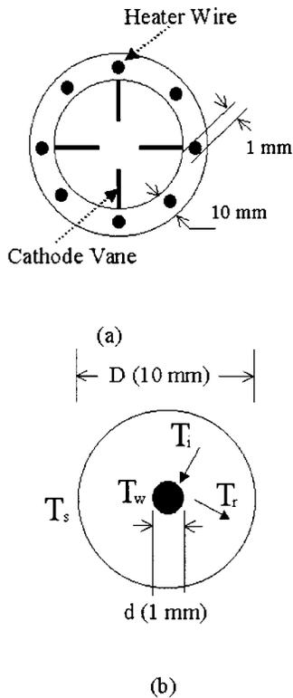
Fig. 2. (a) Cathode structure of ITT F-303 thyatron. (b) Simplified thyatron cathode structure.
