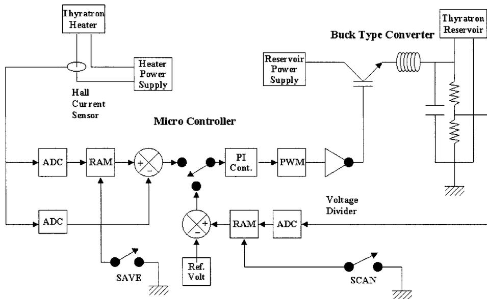
Fig. 7. Circuit diagram of a device for the autoranging and autodiagnosis of thyratron.
