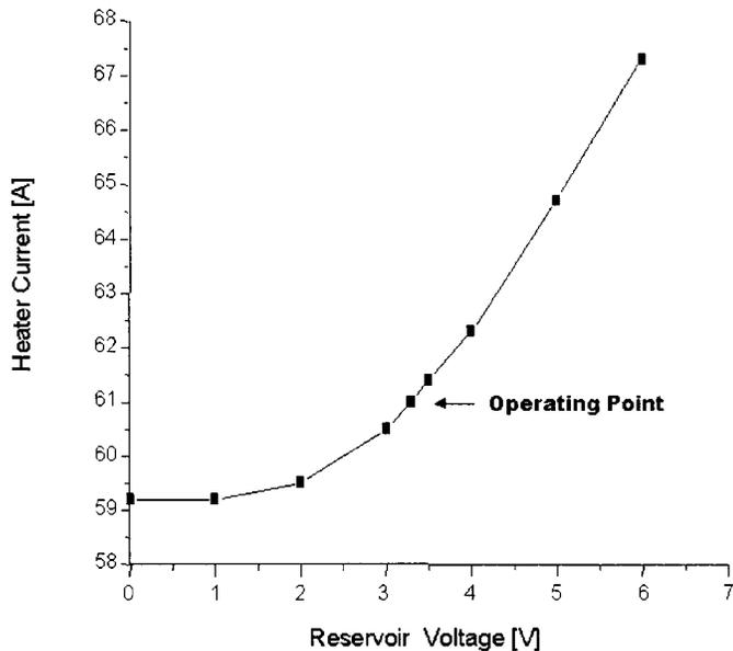
Fig. 5. Plot of a variation of the heater current by changing the reservoir voltage from 0 V to 6 V with a fixed heater voltage of 6.3 V.
