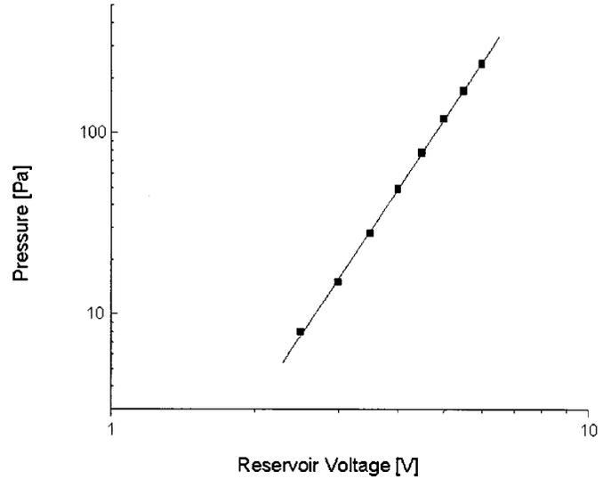
Fig. 3. Variation of the thyratron (ITT F-303) internal gas pressure as the reservoir voltage changes from 2 V to 6 V.
