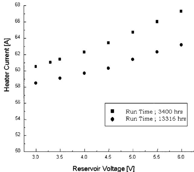
Fig. 6. Comparison of two heater current data as a function of the reservoir voltage for a same thyatron (ITT F-303) measured at a different accumulated high-voltage run-time (3400 h: May 1998, 13 316 h: November 1999). The heater voltage was fixed at 6.3 V.
