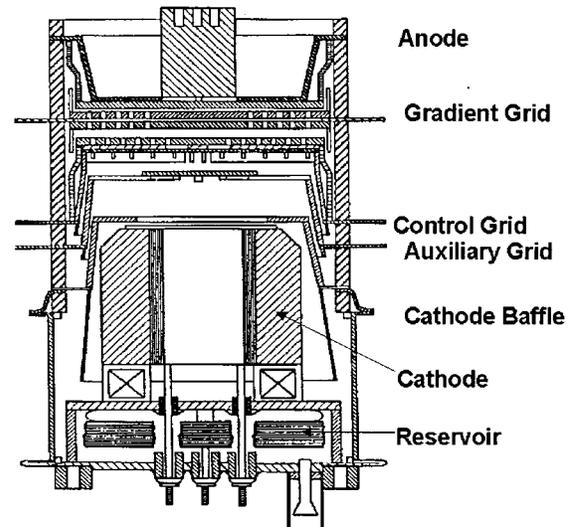
Fig. 1. Typical structure of a thyatron.
