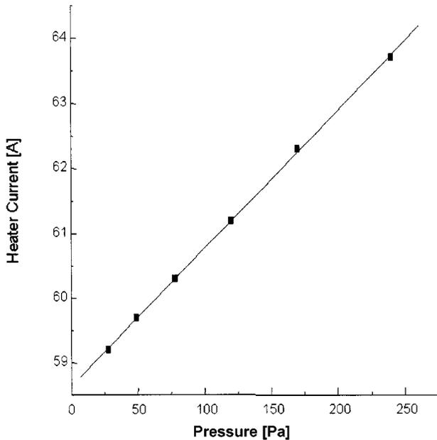
Fig. 4. Variation of the heater current as the internal gas pressure increases from 26 Pa to 240 Pa with a fixed heater voltage of 6.3 V.
