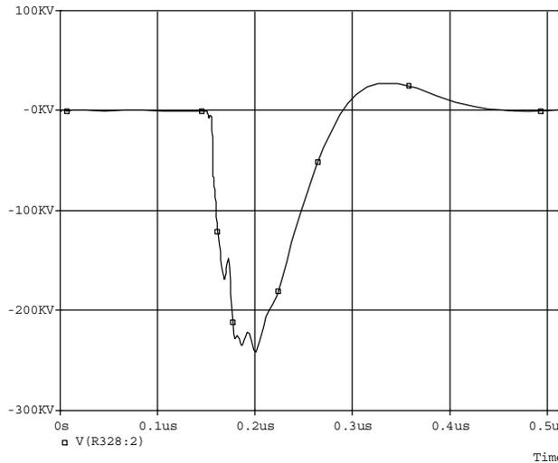
Fig. 6. Modeled result of the Marx generator.
