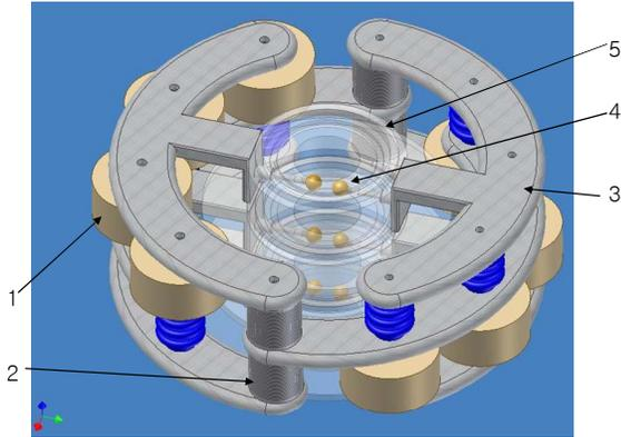
**Fig. 3.** 3D view of the Marx generator. 1: capacitor, 2: charging inductor, 3: guiding connector, 4: spark gap switch, 5: Switch tube
