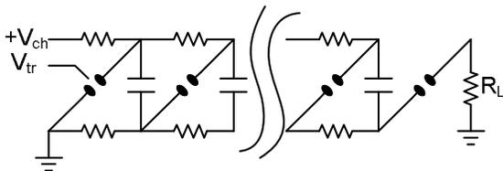
Fig. 1. The basic Marx generator circuit.
