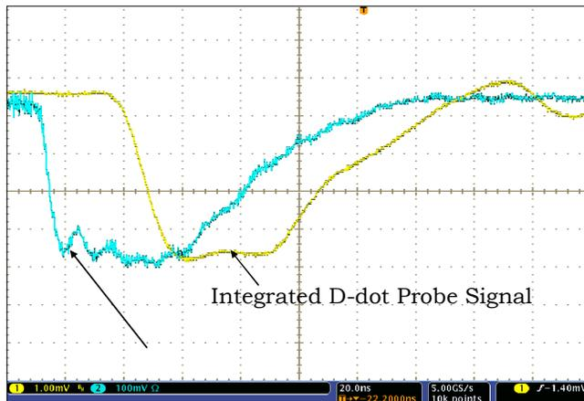
Fig. 7. 100 W aqueous resistor load test result of the Marx generator.
