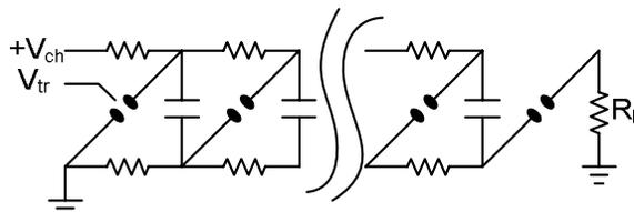
Figure 1. The basic Marx generator circuit.
