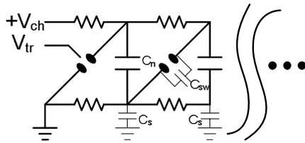
**Figure 2.** The capacitive components in a Marx generator.
