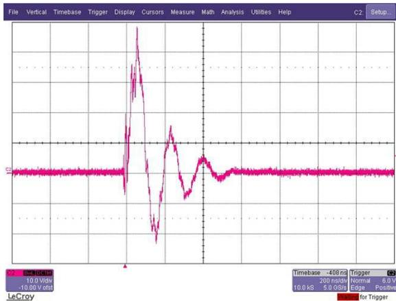
Figure 5. Short circuit current for the Marx generator.
