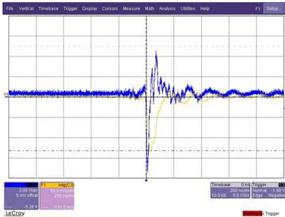
Figure 6. Typical waveform of capacitive voltage probe at 25  $\Omega$  load condition.
