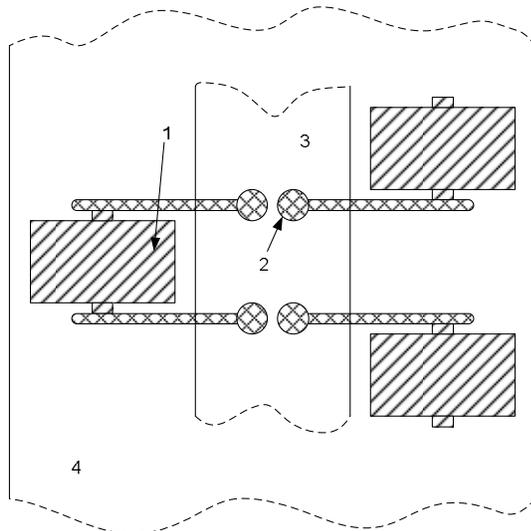
**Figure 3.** Cross-sectional schematic of the Marx generator. (1: Capacitor, 2: Switch, 3: Switch tube, 4: Gas Tank)
