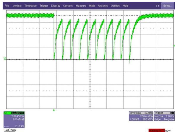
Figure 7. Charging voltage waveform at burst mode operation..
