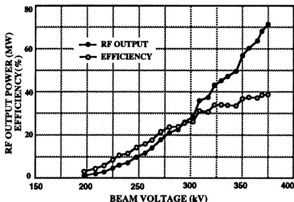
Fig. 1: Plot of beam voltage versus E-3712 klystron RF output power. 150-MW modulator is used to measure the data. (ISOL = 16.5 A, RF drive power = 250W, PRR = 50Hz, Heater power = 440W)
