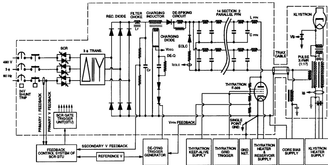
Fig. 2 : Simplified circuit diagram of 200-MW modulator.
