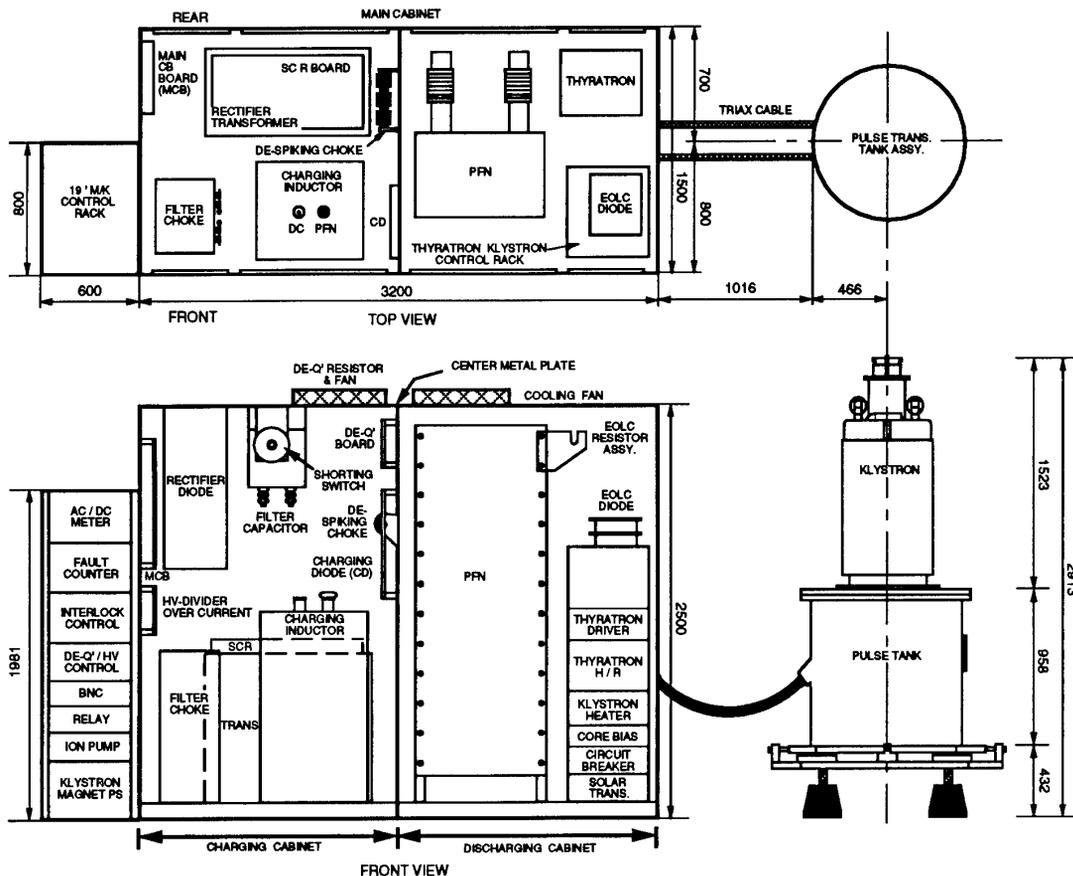
Fig. 3 : Configuration of main components in 200-MW modulator cabinet ( units are in mm).
