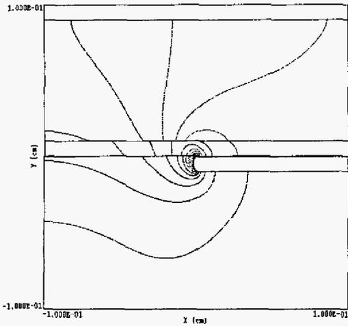
Figure 4(b). The contour plot of electric field for electrode edge (type 1e)
