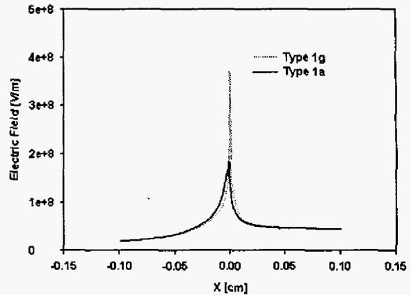
Figure 5. The electric field distribution at  $y = 1.0 \times 10^{-5}$  cm (type 1a, case 6).
