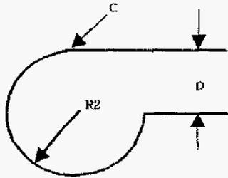
Figure 3. The electrode edge (type 2)
