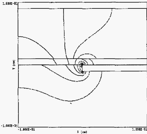
Figure 4(c). The contour plot of electric field for electrode edge (type 1g)
