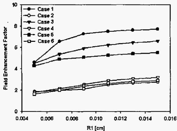
Figure 6(a). Field enhancement factor plot as a function of radius R1 for edge type 1.
