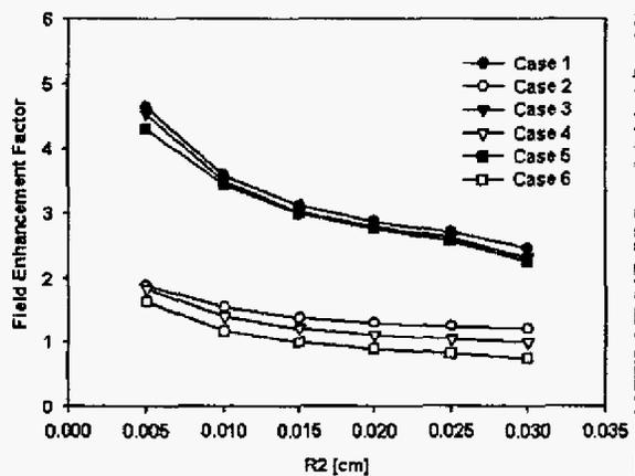
Figure 6(b). Field enhancement factor plot as a function of radius R2 for edge type 2.
