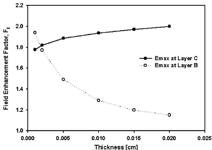
Fig. 11. Field enhancement factor for the edge type R as a function of thickness of the insulation layer C.
