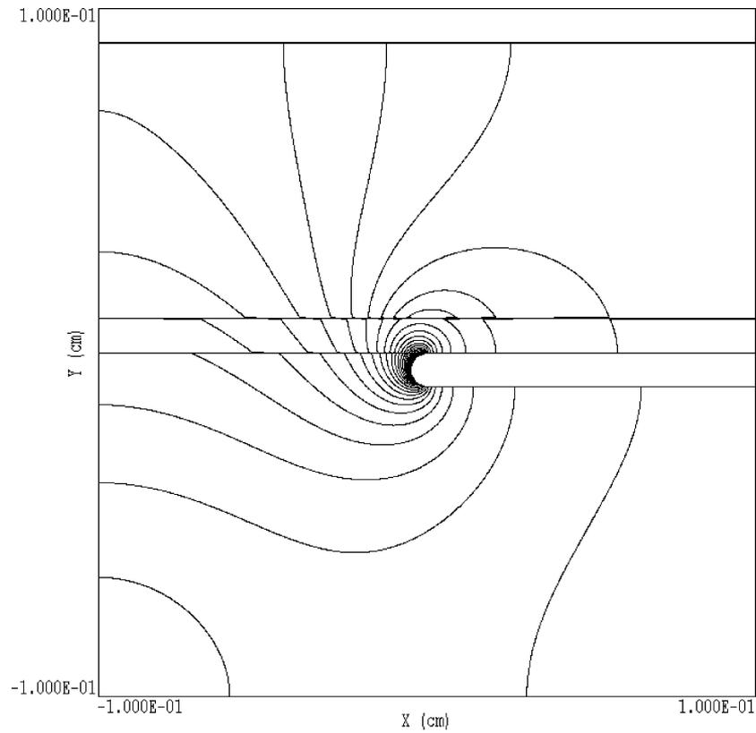
Fig. 4. Electric field distribution for the spiral strip winding edge type-R.
