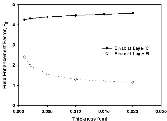
Fig. 12. Field enhancement factor for the edge type S as a function of thickness of the insulation layer C.
