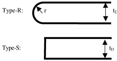
Fig. 3. Shapes of the spiral strip winding edge used in the simulation.
