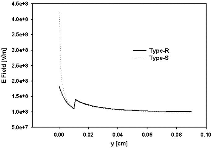
Fig. 6. Electric field distribution in the layers B and C as a function of distance  $y$  ( $\epsilon_{rB} = 3, \epsilon_{rC} = 4$ ).
