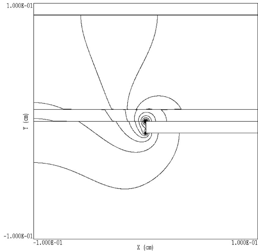
Fig. 5. Electric field distribution for the spiral strip winding edge type-S.
