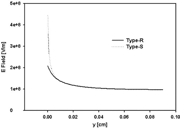
Fig. 7. Electric field distribution in the layers B and C as a function of distance  $y$  ( $\epsilon_{rB} = \epsilon_{rC} = 3$ ).
