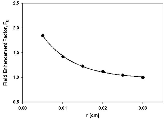
Fig. 8. Field enhancement factor as a function of  $r$  for the type-R case.
