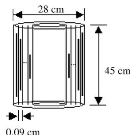
Fig. 1. Schematic drawing of the air cored high voltage spiral strip pulse transformer.
