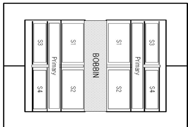
Fig. 6. Type-II winding arrangement of 80-kHz transformer.
