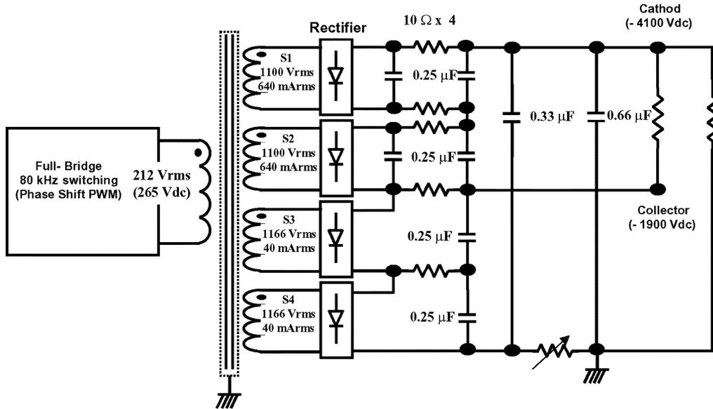
Fig. 2. 80-kHz pulse transformer connection diagram with HV part.
