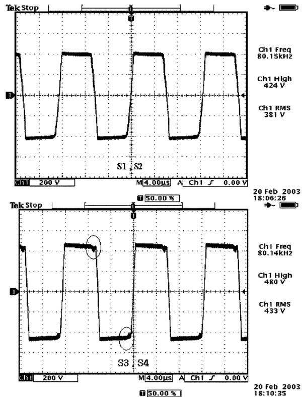
Fig. 9. Output waveforms of 80-kHz type-I transformer.
