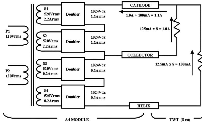
Fig. 1. 100-kHz pulse transformer connection diagram with HV part.
