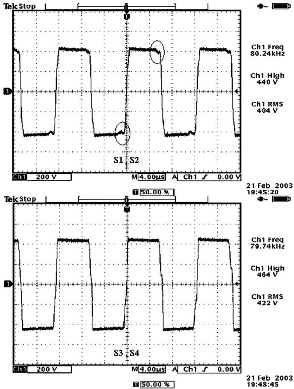
Fig. 11. Output waveforms of 80-kHz type-III transformer.
