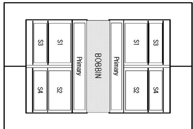
Fig. 5. Type-I winding arrangement of 80-kHz transformer.
