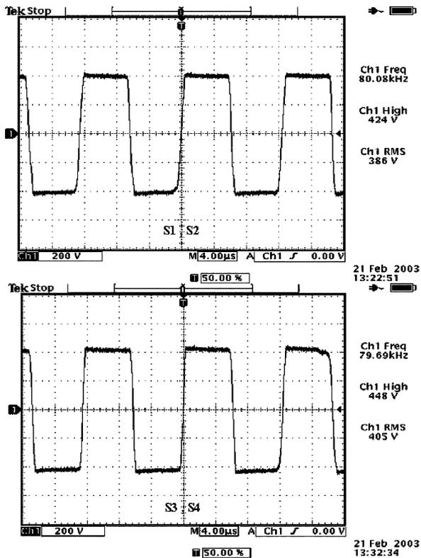
Fig. 10. Output waveforms of 80-kHz type-II transformer.
