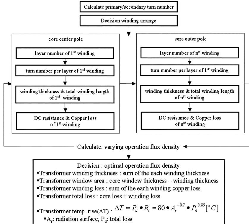
Fig. 3. Transformer winding design procedure.
