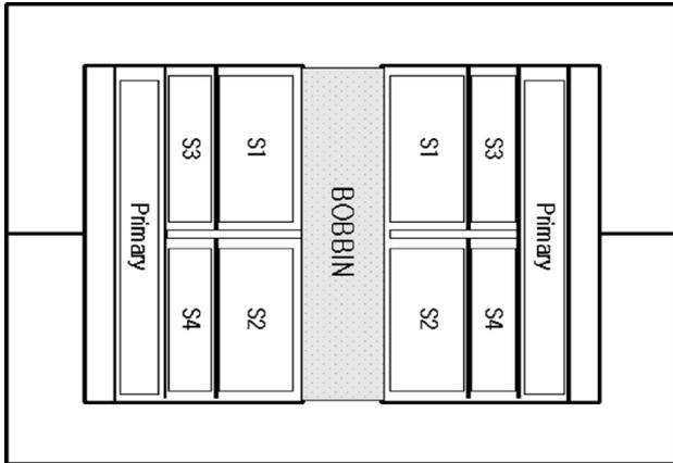
Fig. 7. Type-III winding arrangement of 80-kHz transformer.
