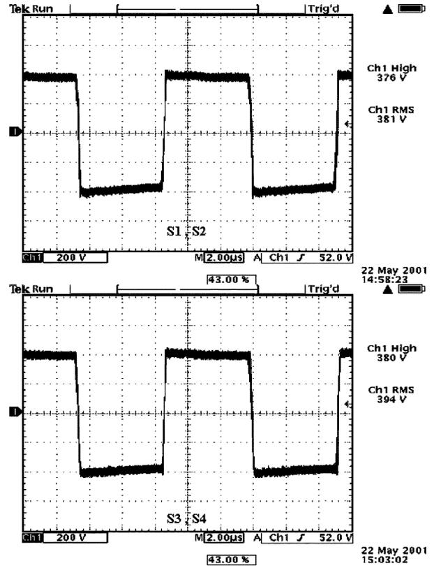
Fig. 8. Output waveforms of 100-kHz transformer.
