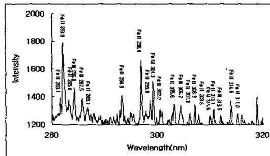
Figure 4. Typical emission spectra of vacuum arc plasma in the Fe electrode TVS in the 280 nm - 320 nm range. The peak current was 64 kA.
