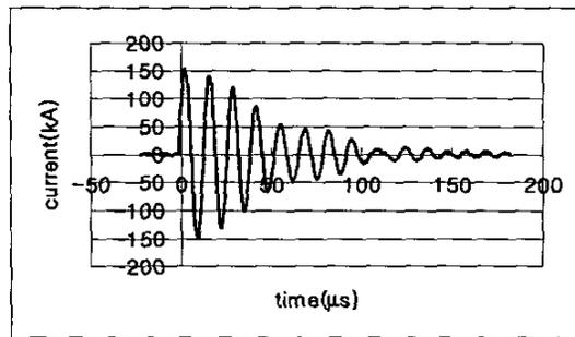
Figure 3. A typical current waveform of the Fe electrode TVS. (150 kA peak with 15 kV charging voltage)
