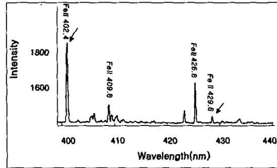
Figure 5. Typical emission spectra of vacuum arc plasma in the Fe electrode TVS in the 400 nm – 440 nm range. The peak current was 64 kA.
