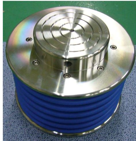
Fig. 2. Prototype spark gap switch.
