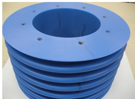
Fig. 8. Cracks are stretched along the outside wall of the corrugated spacer.
