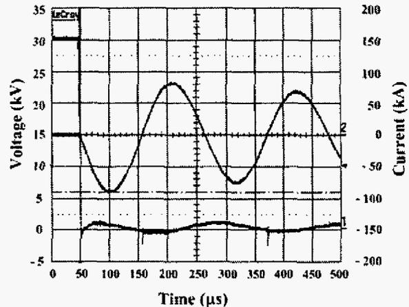
Figure 4. Typical waveforms of voltage(CH1, capacitor charging voltage 30 kVpeak) and current(CH2, 90 kApeak, half-cycle width 100  $\mu s$ ) TVS.
