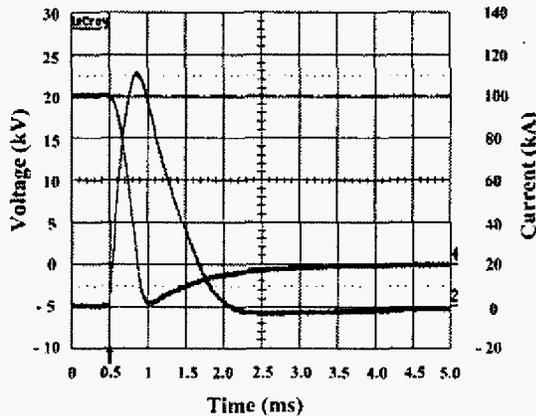
Figure 7. Long pulse test waveforms of voltage (CH1, capacitor charging voltage 20 kVpeak) and switching current (CH2, 109 kApeak). Total switching pulse-width is about 1.5 ms. Transfer charge is 75 C.
