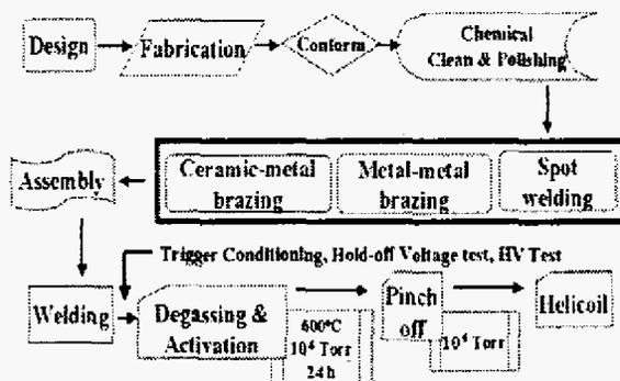
Figure 2. Fabrication procedure of the TVS.
