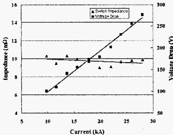
Figure 10. Plot of the switch voltage drop versus peak switch current with  $20 \mu\text{H}$  inductance load.
