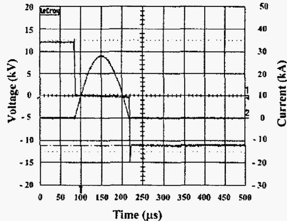
Figure 8. Typical waveforms of the diode phenomenon. (CH1, cross switching voltage 12 kVpeak) and current(CH2, 28 kApeak). Total switching pulse-width is about 134  $\mu$ s.
