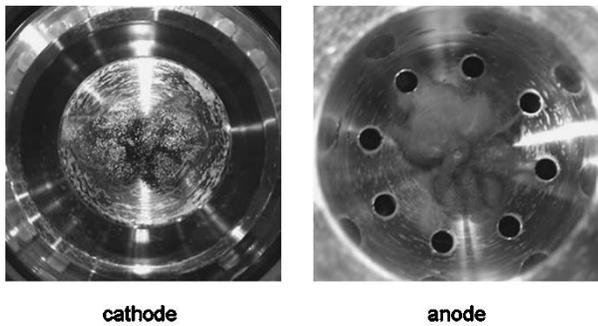
Fig. 10. Photographs of the radial type multichannel pseudospark switch.
