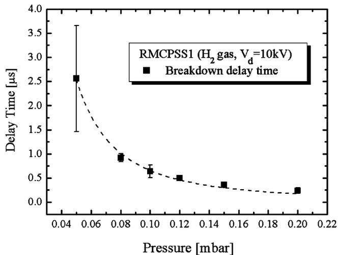
Fig. 5. Measured breakdown delay times as a function of filling gas pressure (hydrogen).
