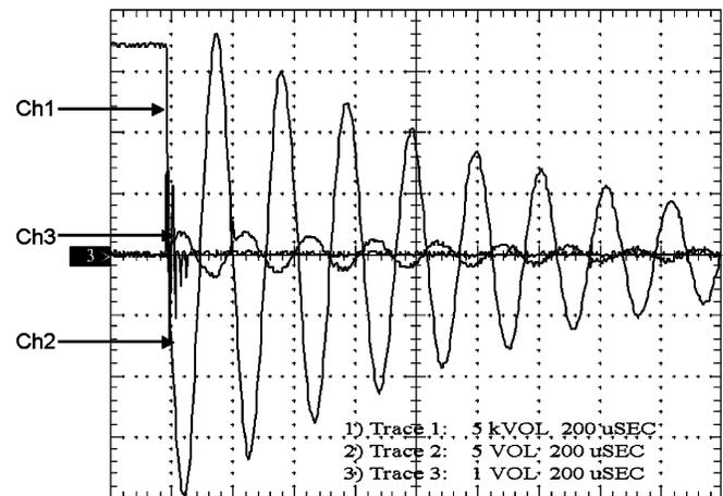
Fig. 13. Voltage and current waveforms of RMCPS2 with a SiC anode disk tested with the circuit in Fig. 12 for He 0.049 mbar and 17 kV. (Peak current: 50 kA. Half period: 100  $\mu$ S.) Ch1: Switch voltage (1 kV/V). Ch2: Switch current (2.5 kA/V). Ch3: Trigger current (40 A/V).
