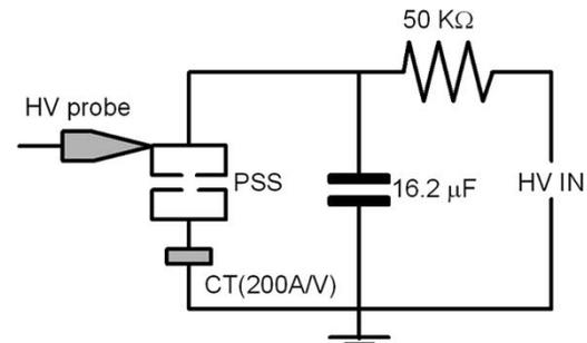
Fig. 7. Circuit used for the high-current test.
