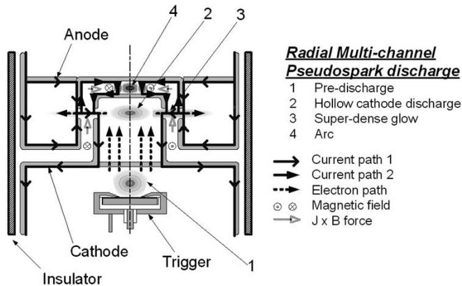
Fig. 1. Discharge process of a radial multichannel pseudospark switch.
