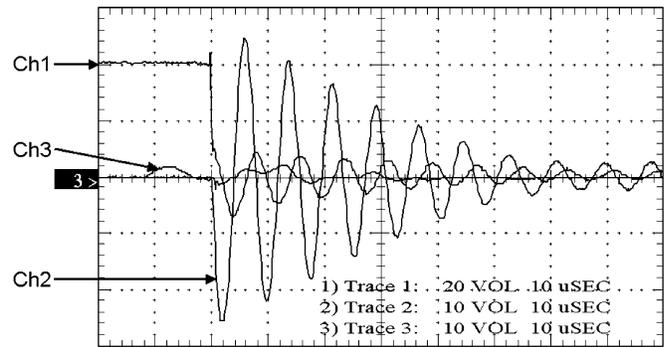
Fig. 11. Typical waveforms of triggered breakdown of RMCPS2 with a SiC anode disk for 0.05 mbar of helium and 20 kV. Ch1: Switch voltage (1 kV/V). Ch2: Switch current (4 kA/V). Ch3: Trigger current (40 A/V).
