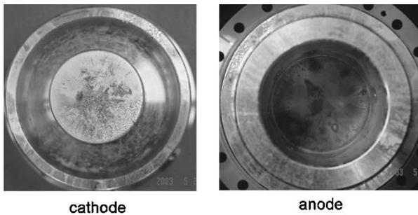
Fig. 14. Photographs of the radial multichannel pseudospark switch, RMCPS2. Right photograph shows the SiC anode disk.
