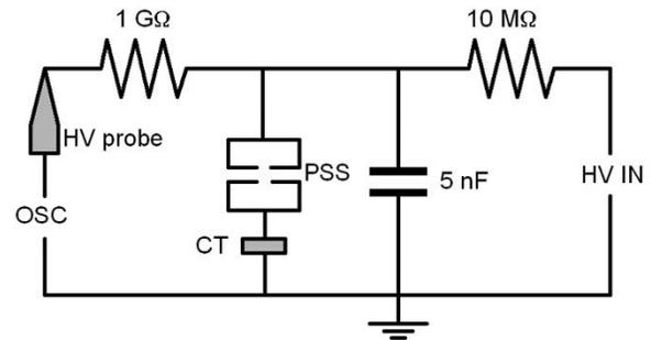
Fig. 3. Circuit diagram of self-breakdown voltage measurement.
