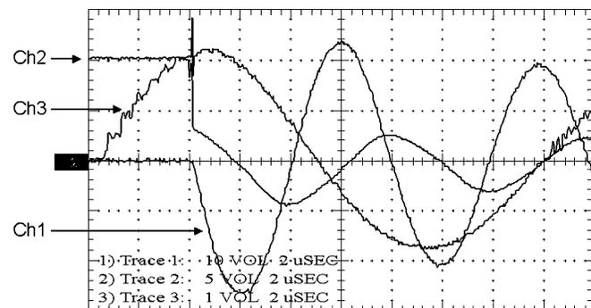
Fig. 8. Typical waveforms of a triggered discharge of RMCPSS2 at  $0.09 \text{ mbar}$  of helium and  $10 \text{ kV}$ . Ch1: Switch current ( $4 \text{ kA/V}$ ). Ch2: Switch voltage ( $1 \text{ kV/V}$ ). Ch3: Trigger current ( $40 \text{ A/V}$ ).
