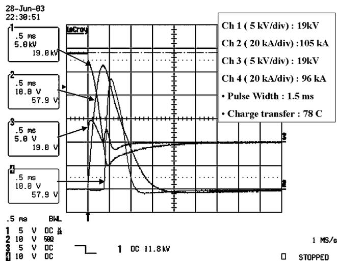
Fig. 15. Typical waveforms for extremely high coulomb-transfer experiments using the test facility of a 300  $\mu$ F capacitor. Ch1: Capacitor voltage. Ch2: Switch current. Ch3: Switch voltage. Ch4: Diode current.
