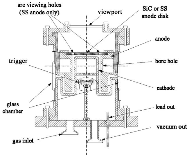
Fig. 2. Schematic of the radial multichannel pseudospark switch, RMCPS2.
