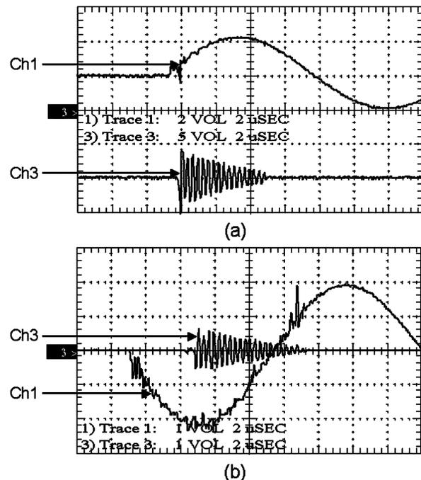
Fig. 6. Typical waveforms of triggered breakdown ( $10 \text{ kV}$ ,  $0.1 \text{ mbar He}$ ). (a) RMCPSS1—Ch1: trigger current ( $40 \text{ A/V}$ ); Ch3: switch current ( $0.2 \text{ kA/V}$ ). (b) RMCPSS2—Ch1: switch current ( $0.2 \text{ kA/V}$ ); Ch3: trigger current ( $40 \text{ A/V}$ ),  $2 \mu\text{s/div}$ .
