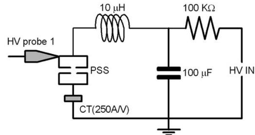
Fig. 12. Circuit for the high-coulomb transfer test.
