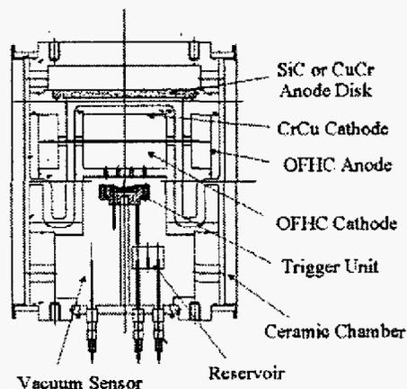
Figure 1. Schematic of the sealed-off radial type pseudospark switch.
