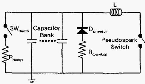
Figure 4. Test circuit of the switch for extremely high coulomb transfer.
